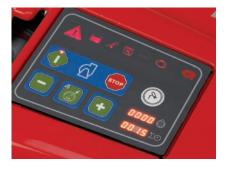
The pump can optionally be controlled via an optional pump pressure governor. The pressure governor automatically keeps the preset pump pressure constant independently of the volume flow of water. Mechanical thermal protection and a cavitation alarm ensure trouble-free operations in any kind of task.
