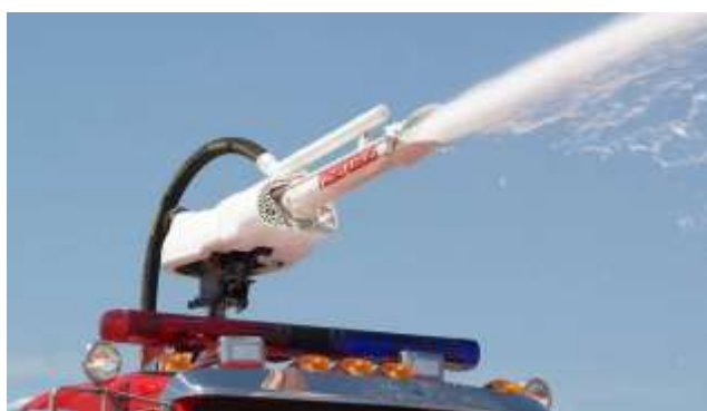
Turret with foam barrel and deflector, on top powder nozzle
