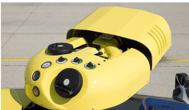
Manual emergency actuation on turret
