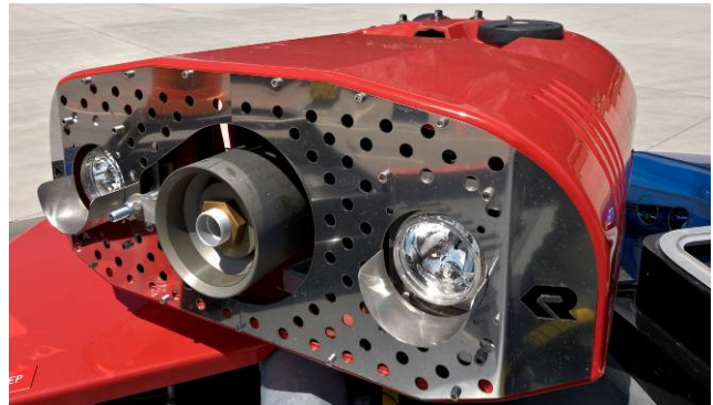
Turret with ChemCore nozzle
