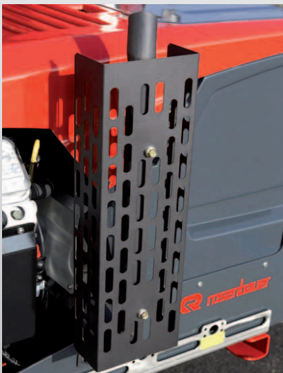
Exhaust gas deflector* for the upward conduction of the gas with turntable ladders
