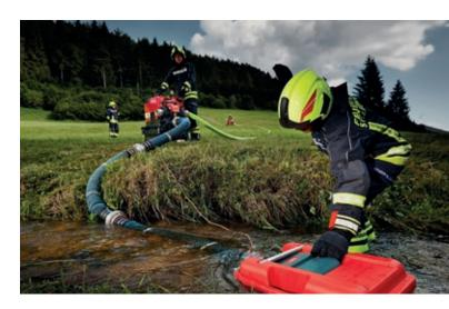
Both portable pumps can be refueled during operation. This is approved and certified by TÜV.
