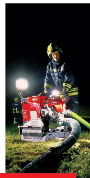
A height-adjustable LED headlight and an optional RLS light head can provide excellent lighting conditions.
